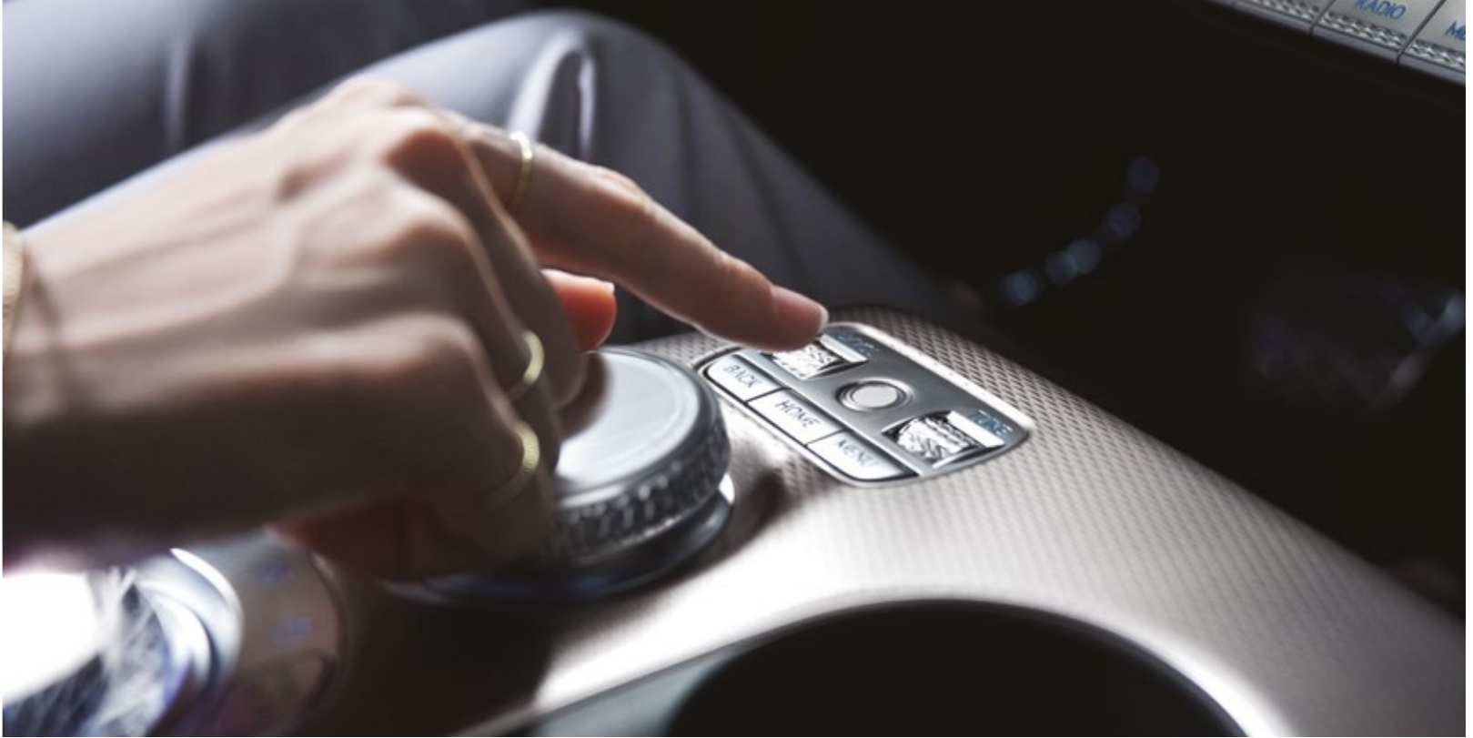
Fingerprint Authentication System _ Allows drivers to access their custom profile.
