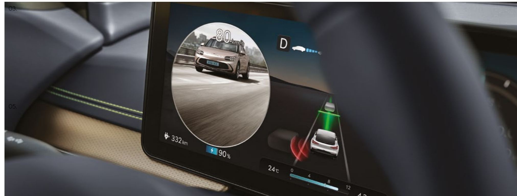
03. Blind-Spot View Monitor (BVM) _ When the driver activates the turn signals to indicate a lane change, video of the respective side and a rear view of the vehicle appears on the center cluster screen.
